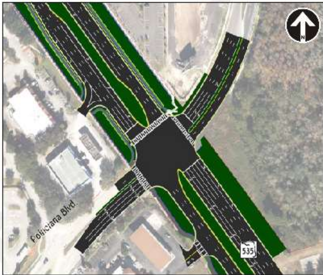
Figure 1-3 SR 535 and Poinciana Blvd Signalized Intersection Alternative
