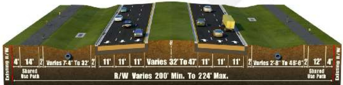
Figure 1-2 Preferred Alternative Typical Section
