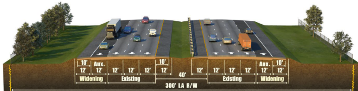
Figure 4. I-75 Typical Section.
