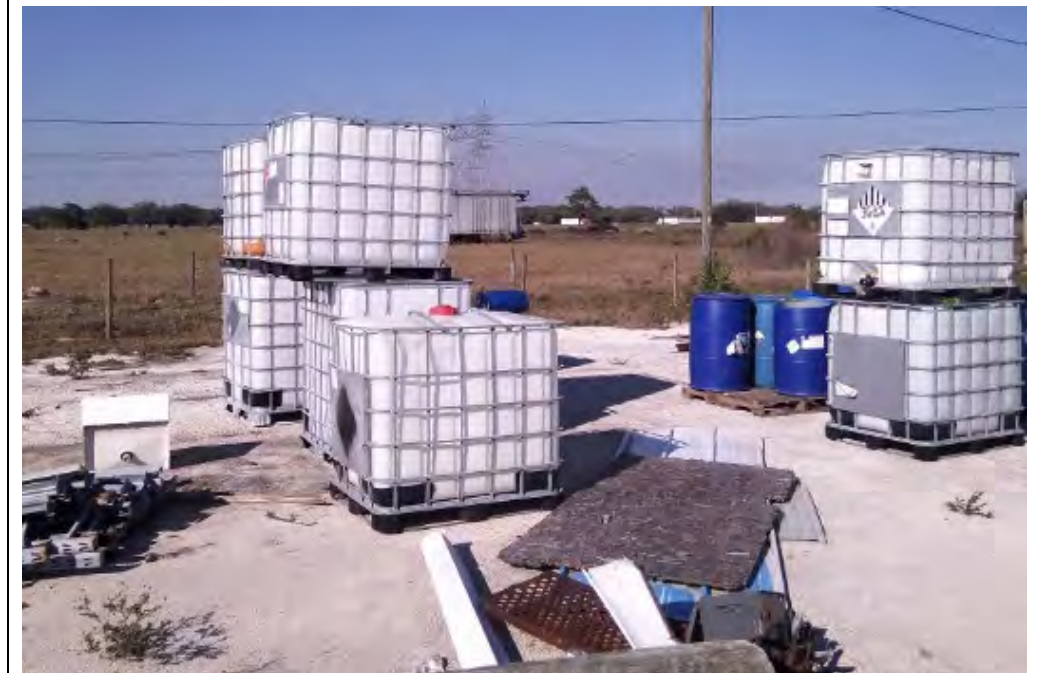
View of seven 250-gallon totes and a pallet of 55-gallon plastic drums.
