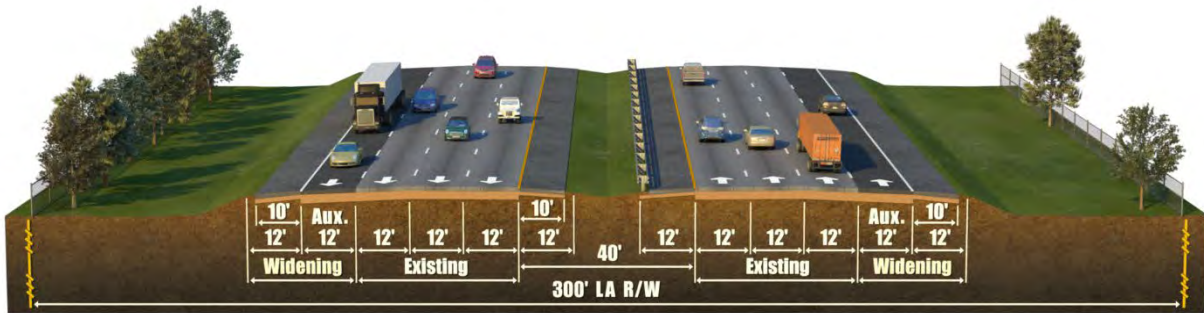
Figure 2.1: I-75 Typical Section
