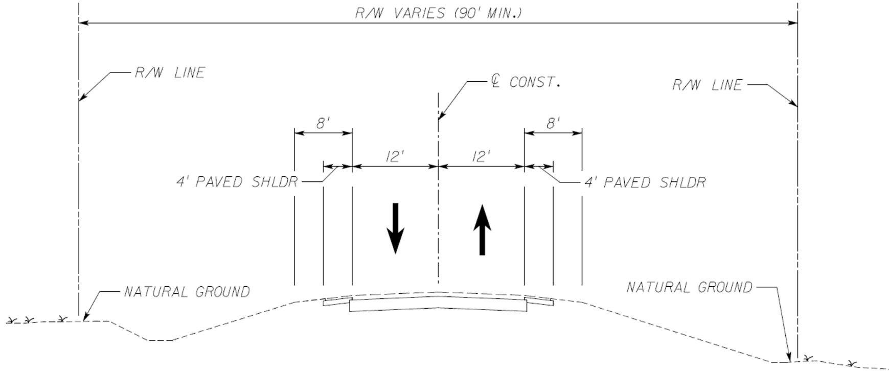
**Figure 2-7 | Existing Typical Section – Segment 5 (Clay Drain Road to Spring Lake Road)**
