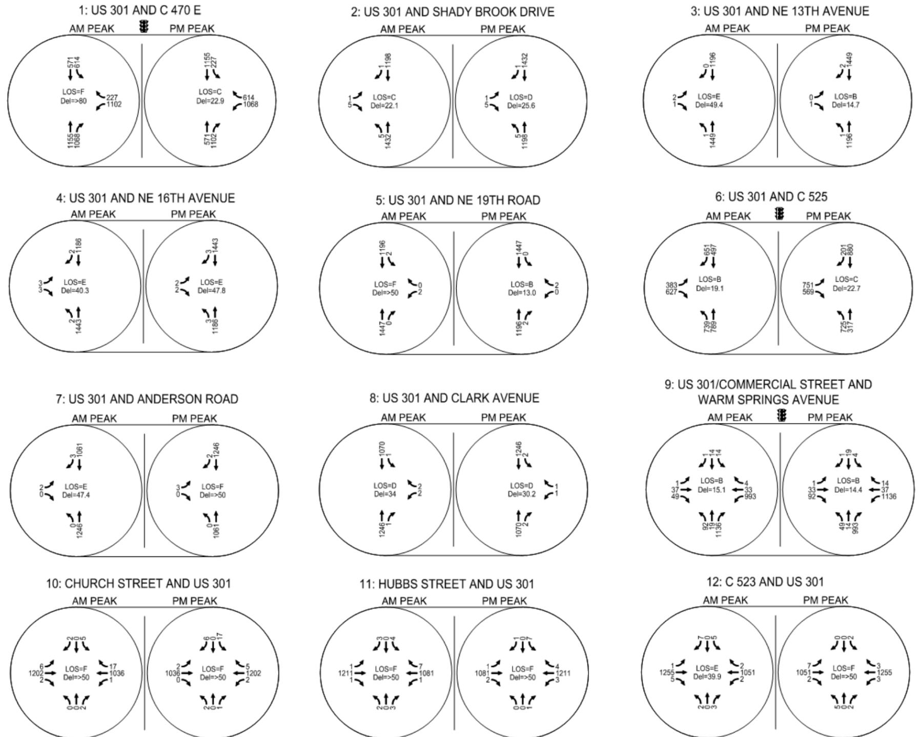
Figure 4-14 | 2042 Alternative 1 – AM/PM Peak-Hour Volumes and LOS – Part B
