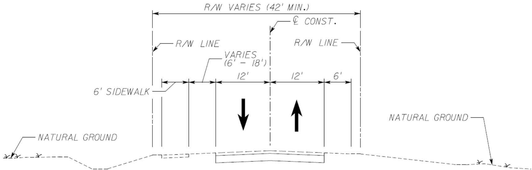
**Figure 2-6 | Existing Typical Section – Segment 4 (Stokes Street to Florida’s Turnpike)**
