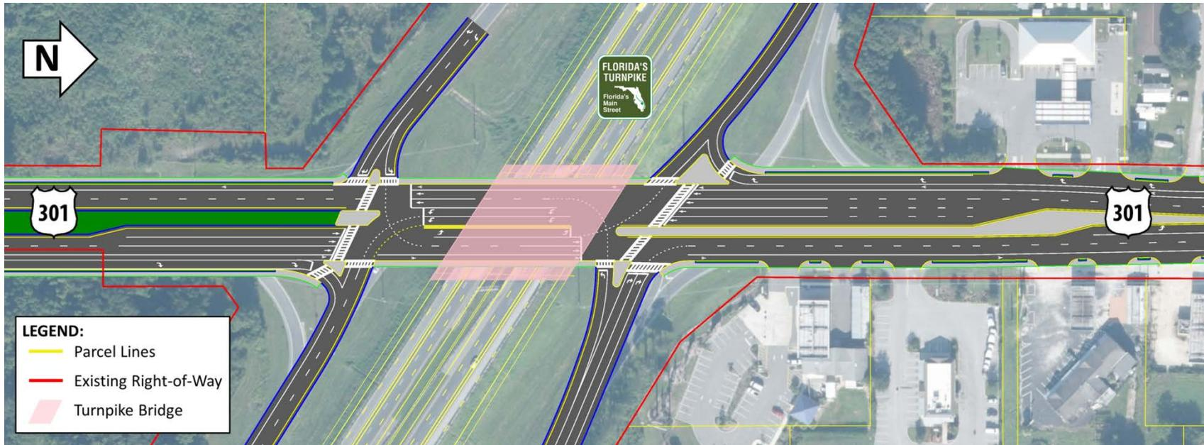
**Figure 4-24 | Diverging Diamond Interchange Configuration**
