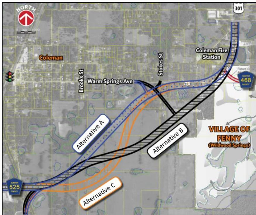
Regarding the realignment alternatives, the consensus communicated to the Project Team by the public was a preference for both Alternative B and Alternative C. It was also identified that there is concern about potential realignment alternatives or the US 301 mainline widening impacting the Coleman Oaks subdivision community well and septic system located on the west side of US 301, north of the CR 468 intersection.
