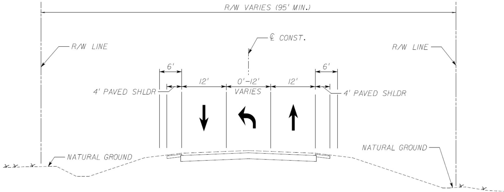
**Figure 2-3 | Existing Typical Section – Segment 2 (Shady Brook Drive to CR 525 E) and Segment 3 (CR 525 E to Anderson Road)**
