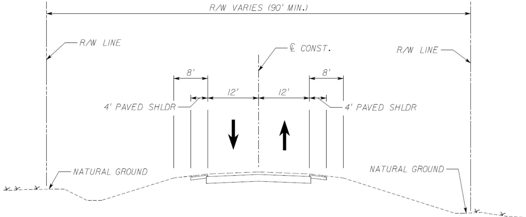
**Figure 2-4 | Existing Typical Section – Segment 3 (Anderson Road to Warm Springs Avenue)**
