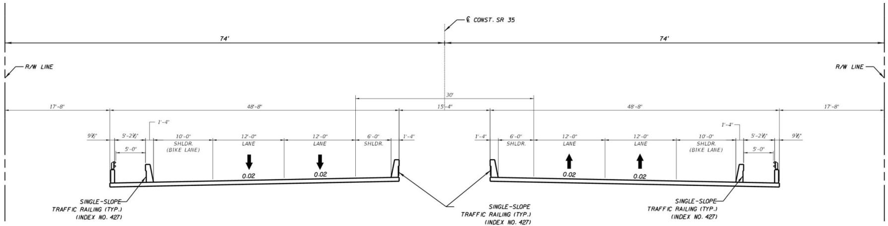
**Figure 4-22 | Bridge Alternative 3 – Typical Section**
