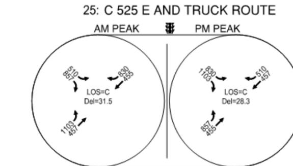
Figure 4-17 | 2042 Alternative 2 – AM/PM Peak-Hour Volumes and LOS – Part B
