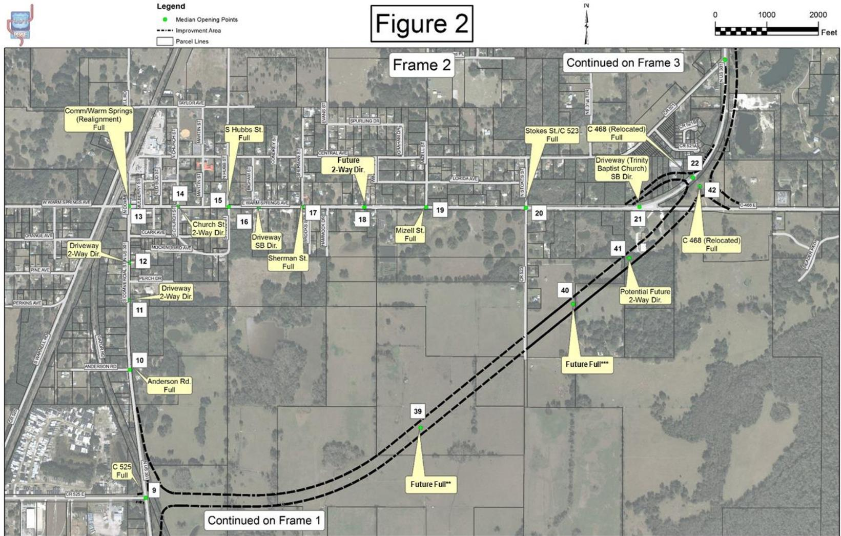
\*\*To be constructed as Full Openings in order to allow access and U-turns to adjacent residences south of the new alignment. Left turn lanes do not need to be constructed initially just to serve these individual residences.
