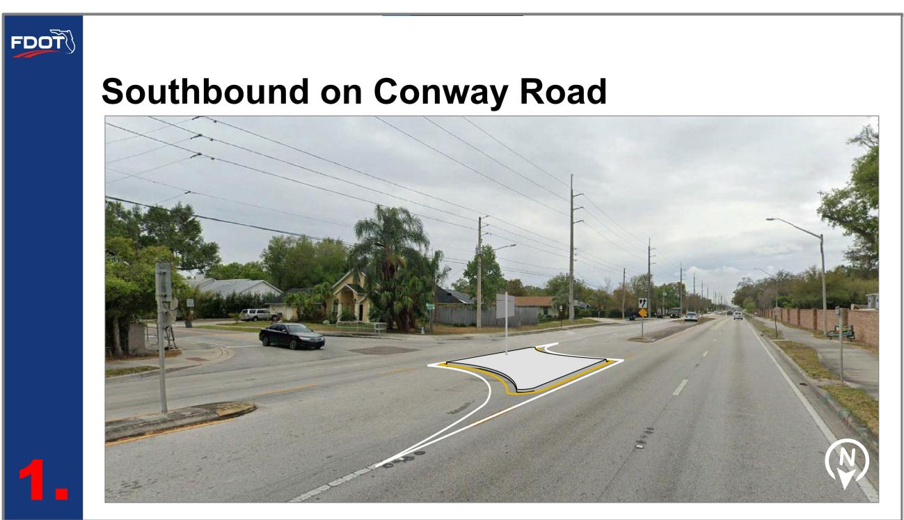
Proposed improvements looking southbound on Conway Road, including the construction of a median island, creating a bi-directional median opening.
