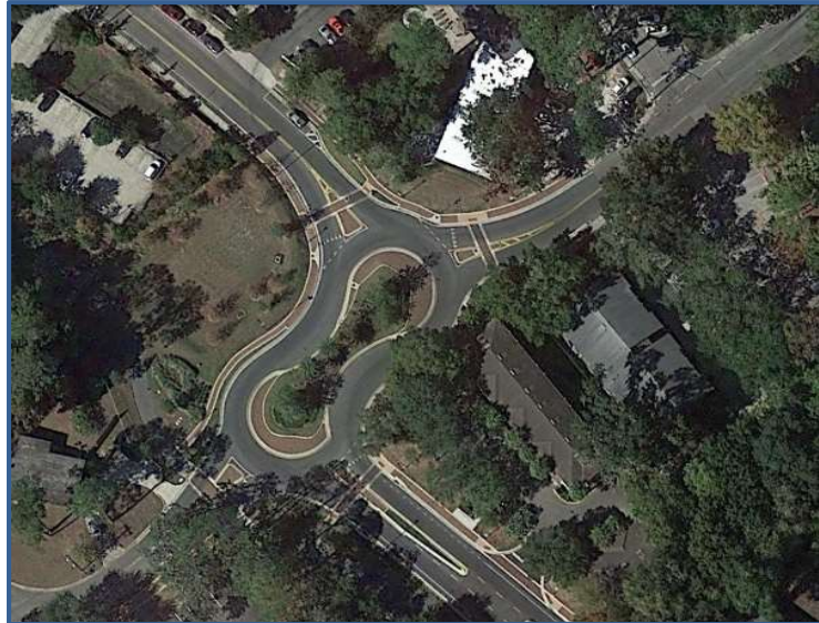
The SW Depot Avenue at 11 th Street Roundabout, in Gainesville, FL, is an example of a roundabout designed in a “peanut” or “dog bone” configuration. (Google Earth)
