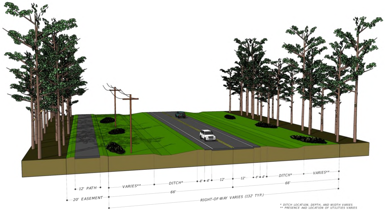
Figure 8 | Typical Section 2 – Trail in Separate Easement
