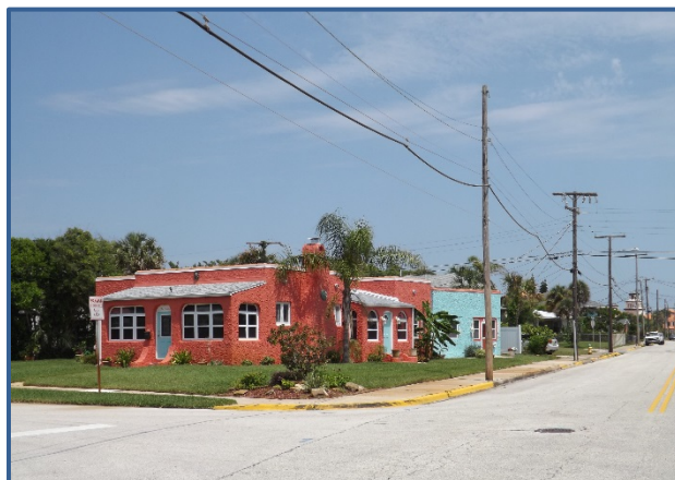
A corner lacking ADA accessible sidewalk ramps at the intersection of Grandview Ave and Ribault Ave.
