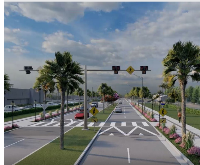
Midblock crossing with pedestrian signal (pedestrian hybrid beacon)
