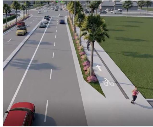
Separated bicycle lane and sidewalk
