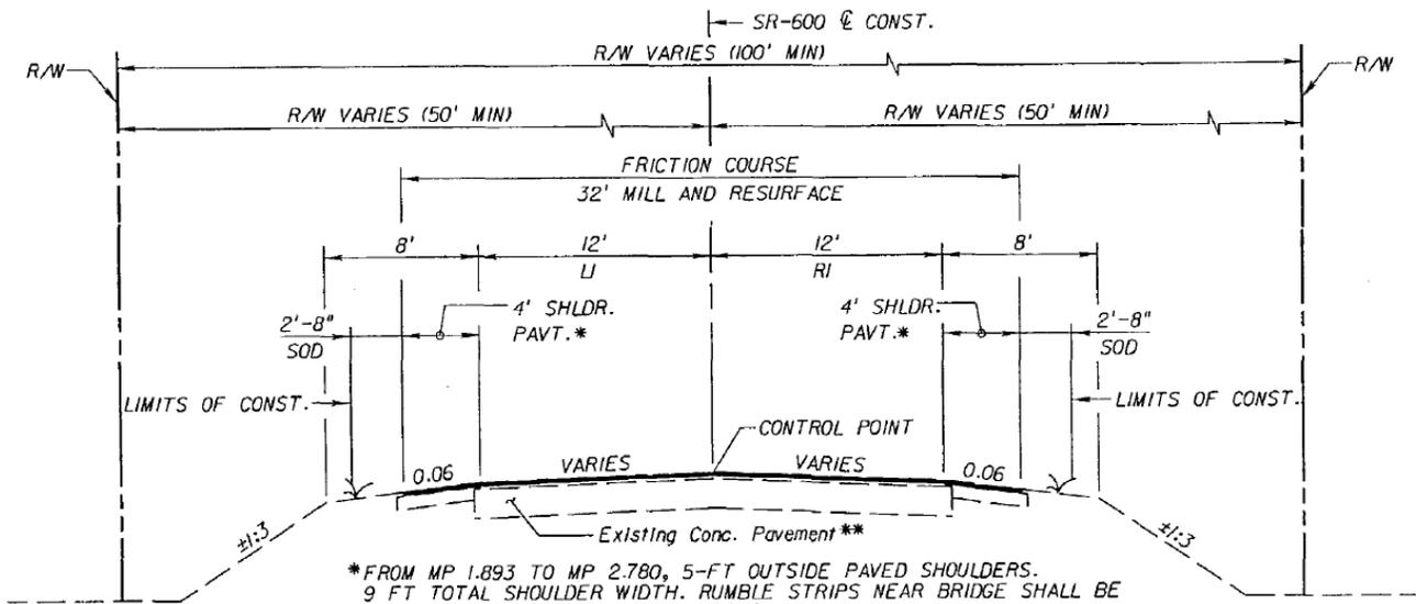
\*FROM MP 1.893 TO MP 2.780, 5-FT OUTSIDE PAVED SHOULDERS. 9 FT TOTAL SHOULDER WIDTH. RUMBLE STRIPS NEAR BRIDGE SHALL BE RECONSTRUCTED AT EXACT LOCATIONS.
