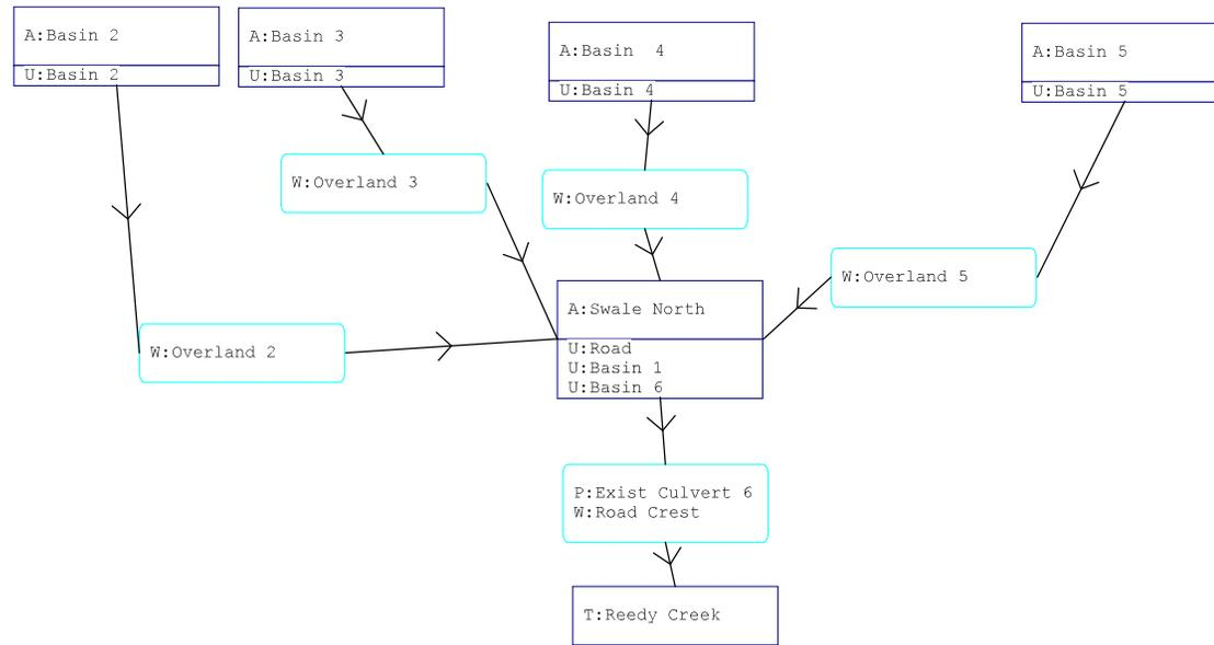
Name: Exist Culvert 6      From Node: Swale North      Length(ft): 85.00
